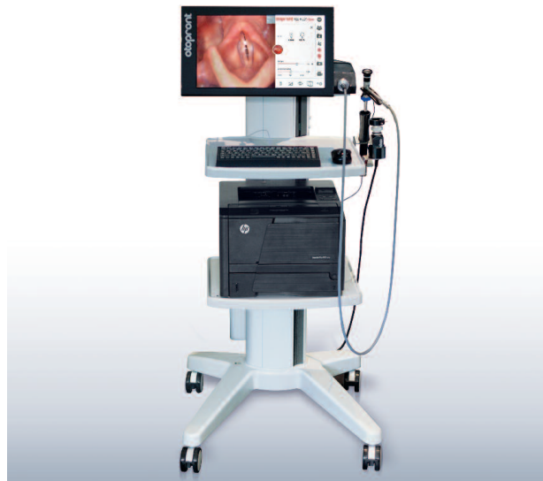
The picture shows the stroboscope on a trolley with printer and storage quivers for endoscopes
